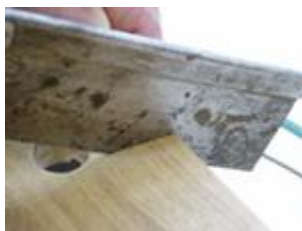
4. Cut neatly down the lines with a fine tooth saw.
